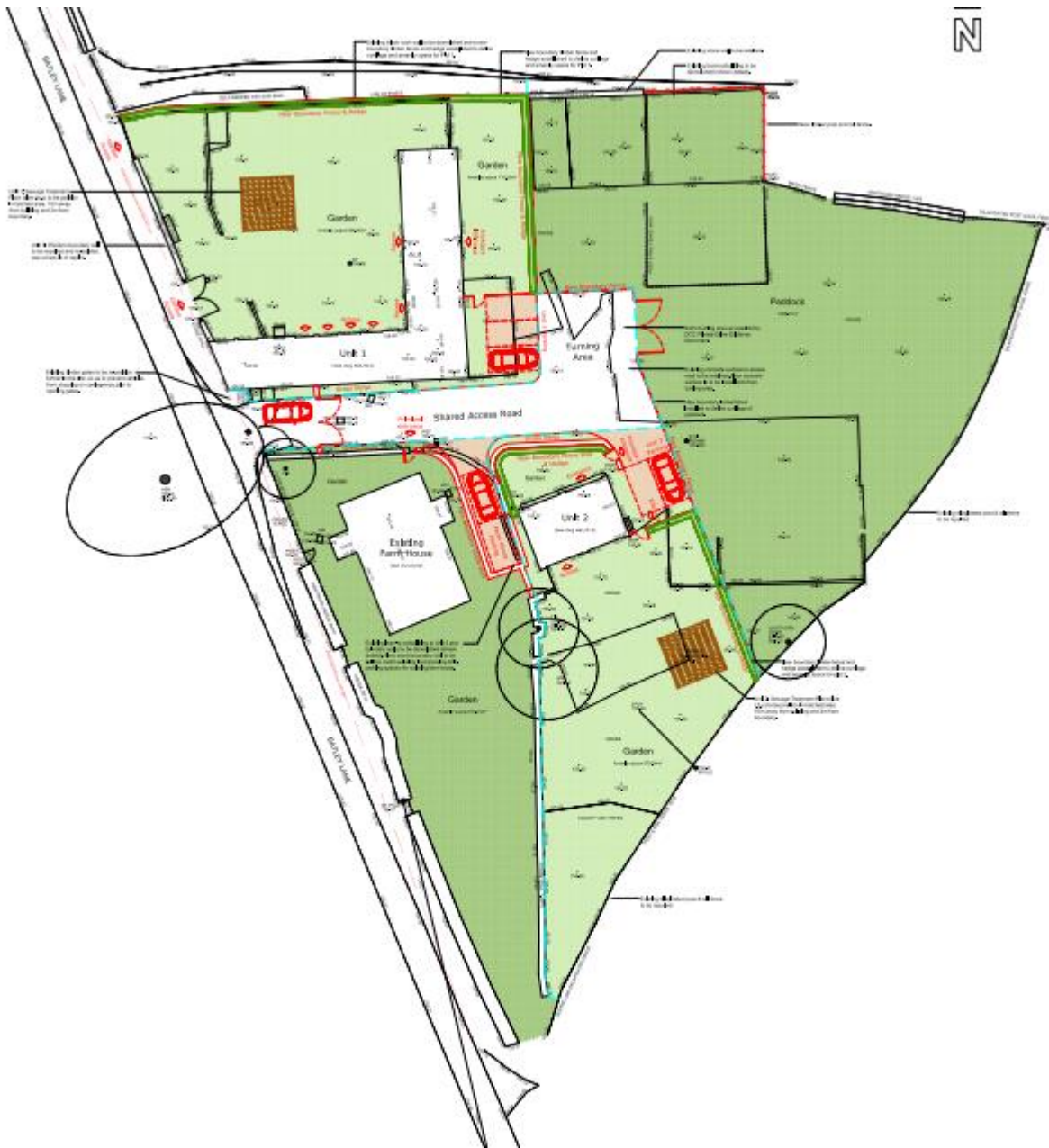
The approved site layout drawing no 011 Rev C defining the approved garden curtilages of each dwelling in light green and excluding the paddock and farm buildings from garden in dark green to the north-east.
